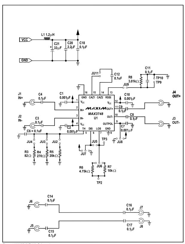
Figure 1 MAX3748 EV Kit Schematic.
