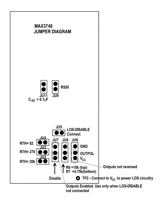
Figure 2. Jumper Diagram.
