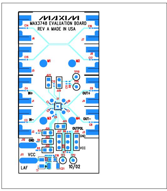
Figure 3. MAX3748 EV Kit Component Placement Guide – Component Side (2X)
